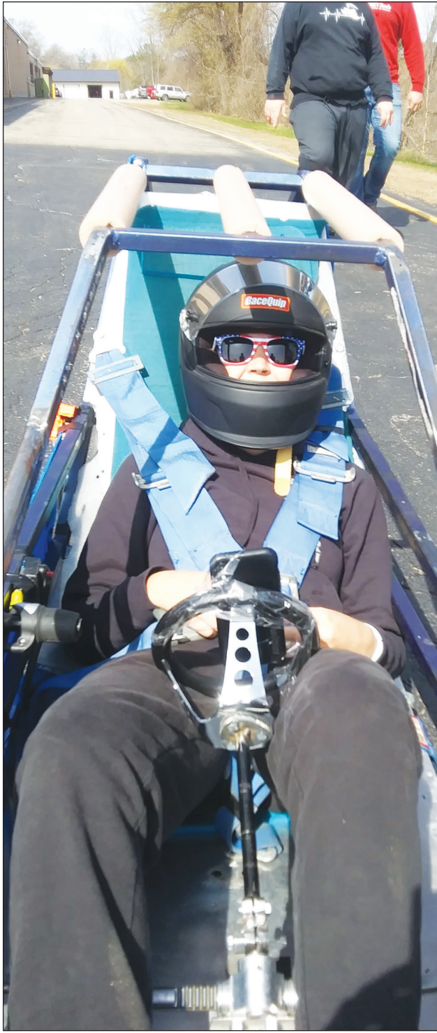
Special to the EagleHerald Georgia Lacroix sits ready to test Peshtigo's electric car in preparation for the upcoming race season. Each car must have padding and a five-point harness.
